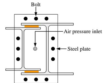
(b) Upper view of test apparatus
