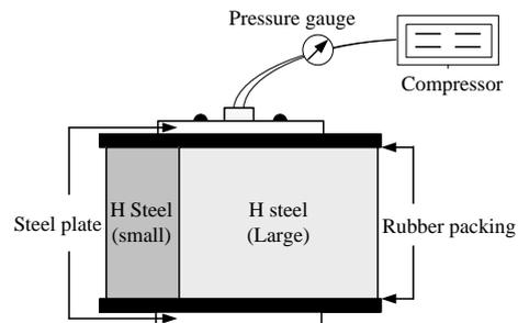
(c) Side view of test apparatus
