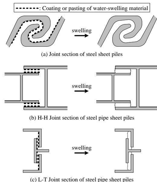
Figure 1. Water cut-off treatment on joint section of steel sheet piles or steel pipe sheet using water swelling materials
