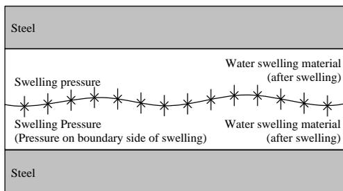
Figure 4. Image of swelling pressure on swelling boundary side
